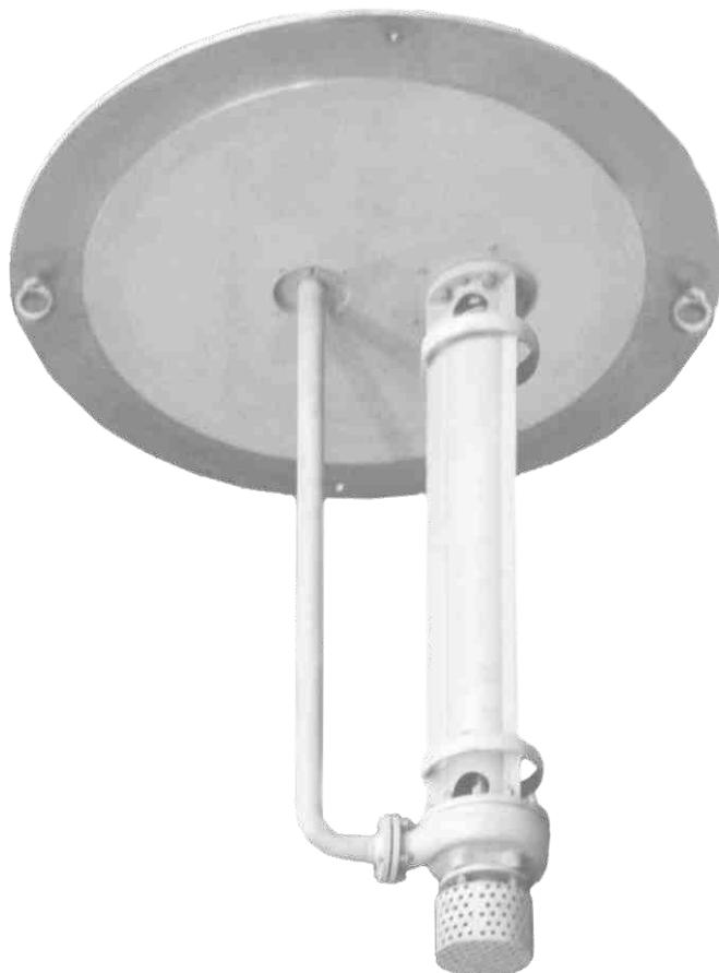
Submerged pumps and pumping units on their basis are designed for pumping of weak aggressive and neutral liquids with density of no more than  $1050 \text{ kg/m}^3$ , containing solid impurities up to 0.2 mm and volume concentration no more than 1.5 %.
