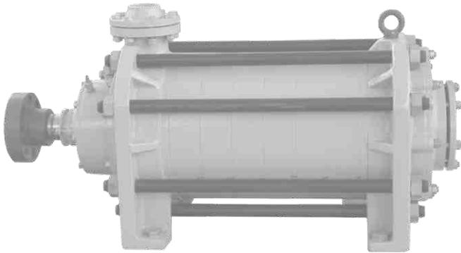
Pumps and electric pumping units of CNS type with the capacity of 40, 80, 200 m<sup>3</sup>/hour and head from 90 to 425 m are designed for pumping of pure and contaminated water with the following properties:
