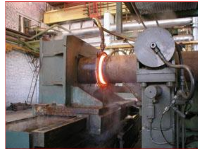
Pipes bending at HFC heating machines
