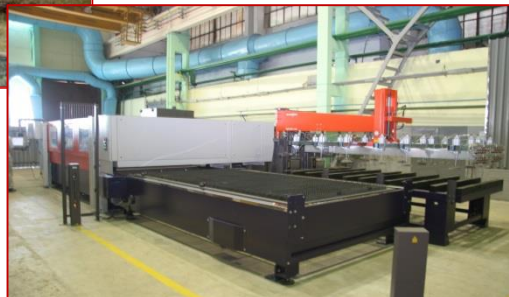
Bystronic Bystar 4020 metal laser pattern cutting machine
