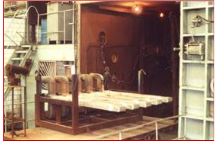
Electron-beam machine for oversized products welding:
