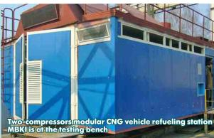
Process equipment of one-and two-compressors modular CNG vehicle refueling stations are operated in climatic zones with ambient temperature from -50°C to +45°C and in regions with seismicity up to 6 on the Richter scale.
