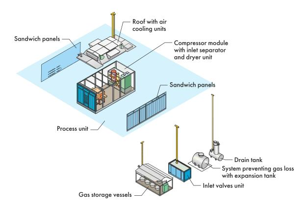
For enhancement of one-compressor station functional capacities, the Company offers the following set of equipment:
