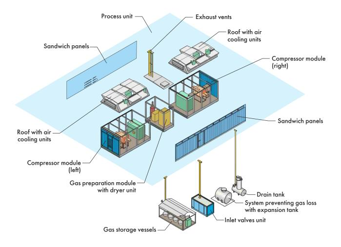
For enhancement of two-compressors station functional capacities, the Company offers the following set of equipment:
