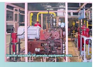
Before shipping to the Client each product undergoes acceptance tests on natural gas under operating conditions.
