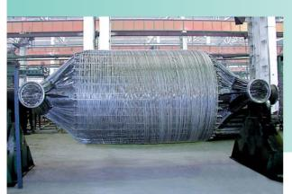
The equipment is being worked out for individual projects and can be made of carbon, corrosion-resistant steels, titanium alloys and nickel-base alloys (Hastelloy "C" type).
