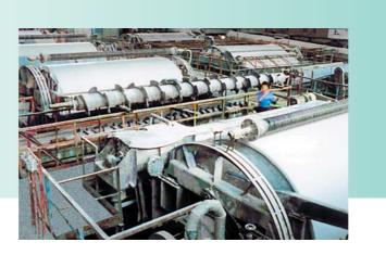
The drum vacuum filters are designed for filtration of difficult to filtrate suspensions in titanium dioxide production (BBM45-3.14-1G), of sodium bicarbonate suspension in soda ash production (BB-5.4 and BYaN-180) as well as in other chemical productions.
