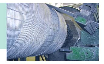
Equipment for mechanized manufacturing with the help of rolling methods of  $5,000 \text{ m}^3$ ,  $10,000 \text{ m}^3$  and  $20,000 \text{ m}^3$  tanks has been designed, manufactured and applied at the enterprise.
